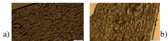
Figure 1. Cross-section of 3D printed tablet a) before and b) after dissolution
