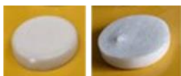
Fig. 1. Lyophilizates with gelatin: PVP K25: glycine/ croscarmellose: mannitol = 0.5: 2: 0.5: 4.5 (glycine left, croscarmellose right).
