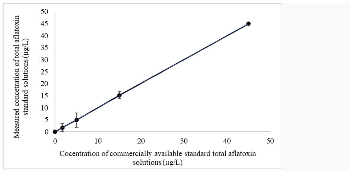
Fig. 2. A calibration curve plotted using five ready-to-use standard solutions of aflatoxins in methanol:water mixture (70:30 v/v) at a given concentrations of 0, 1.7, 5, 15, and 45 µg/L and corresponding measured concentrations.
