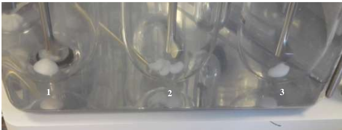
Fig. 2. Dissolution behavior of reference product during sampling intervals in hemispheric vessel, (1, 3- adhered mound; 2 - displaced mound).
