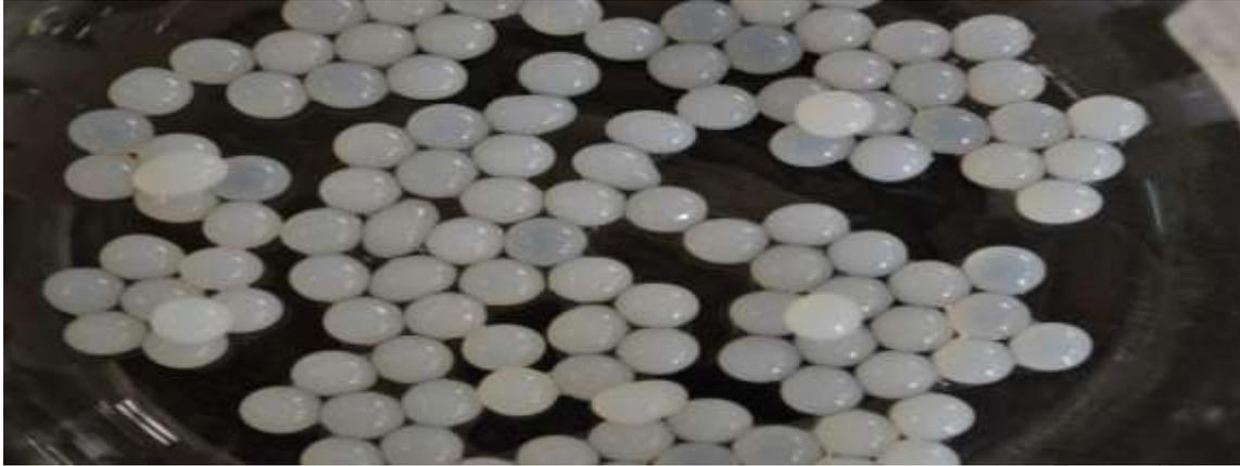
Fig. 4. Appearance of the alginate beads with entrapped enzymes.
